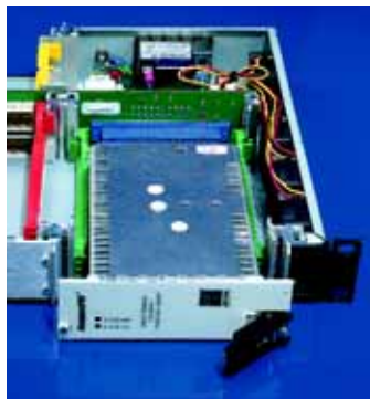
. . . optional plug-in power supply (hot swap capability).
